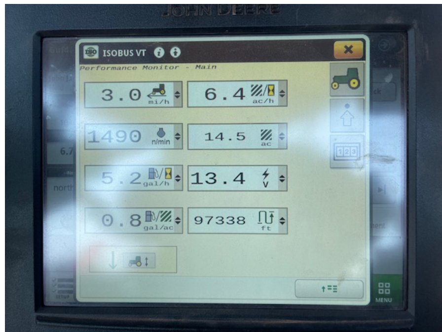
Fig 1: In cab fuel consumption monitor; gal/hour parameter used for GHG emission calculations gcs2023
