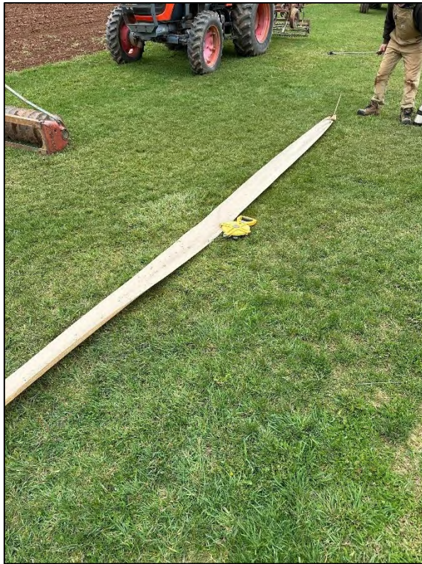
Test strip of paper towel to replicate precise product placement by hand boom
