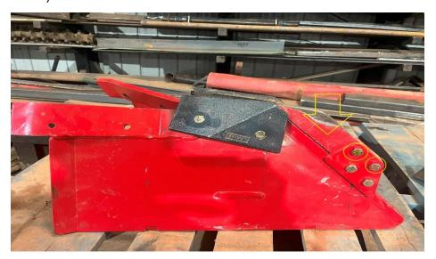
Use a torch or plasma cutter to remove the tab circled below. Then use a grinder to smooth the cut and make sure it is level with the bottom of the shoe. This can be done with the black cast iron wear plates still installed.
