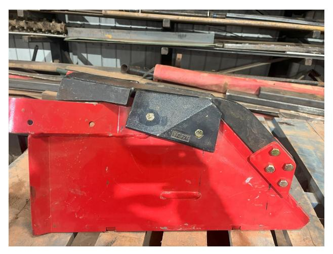
First you will need to remove the two 7/16 bolts circled in yellow below. Loosed the other two as well and then remove the original front wear plate.(indicated by yellow arrow)
