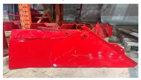
To install the new Furrow Bottom Wear Plate, bolt it loosely in place 7/16x2 bolts and locknuts. Make sure that it is even with the bottom of the shoe and will make a smooth furrow bottom. Remove more material with grinder if needed. Tighten locknuts when the fit is satisfactory.
